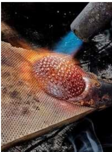
Fig 17: Granulation process — copper spherules applied to the rounded neckpiece element
