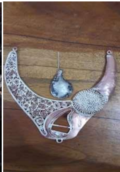
Fig 18: Major parts of bridal necklace after soldering
