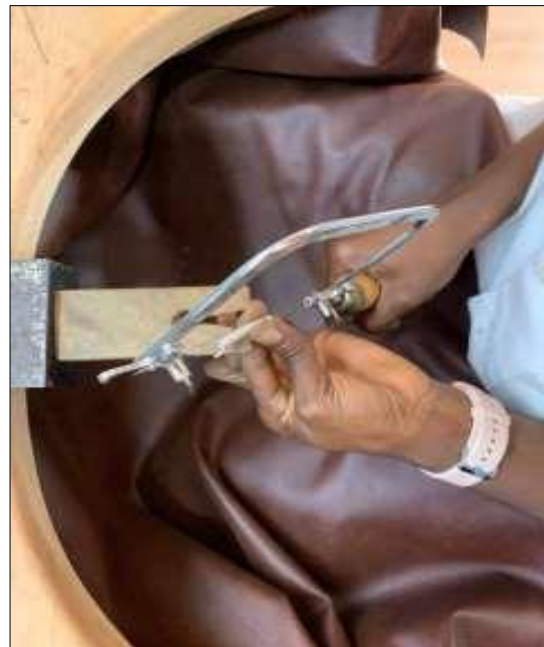
Fig 8: Cutting coiled silver wires into jump rings
