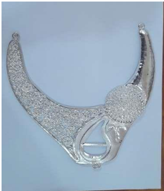
Fig 20: Copper main neckpiece after silver plating
