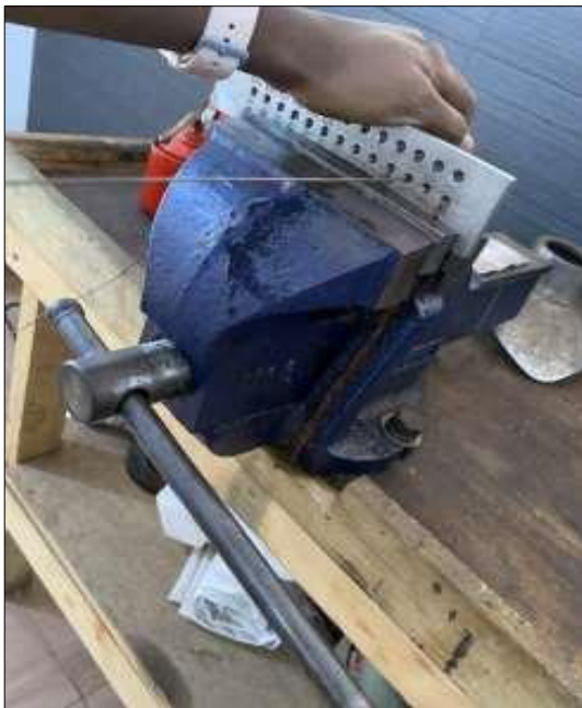
Fig 7: Drawing silver wires to gauge
