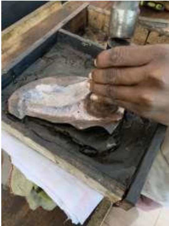
Fig 10: Chasing the main neckpiece
