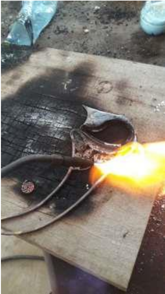
Fig 15: Soldering filigree parts into the neckpiece framework
