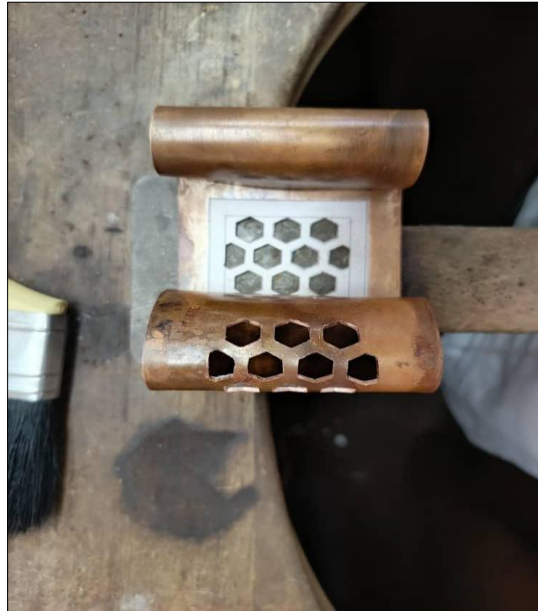
Fig 6: Piercing out the hexagonal shapes (Studio work, 2025)
