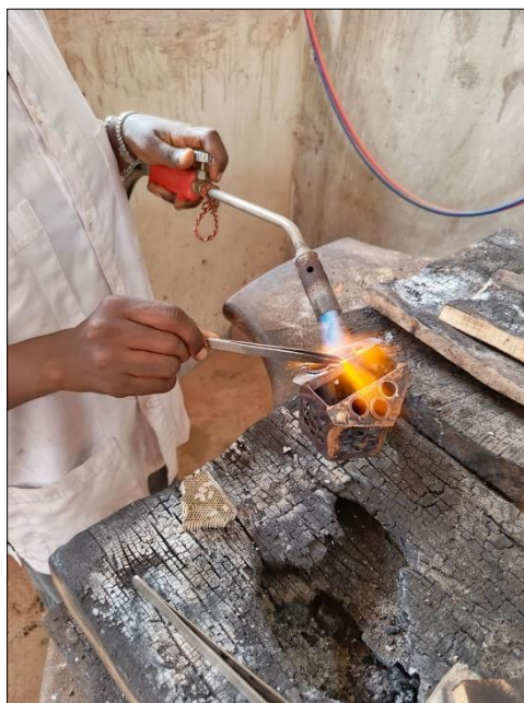
Fig 17: Soldering attachments and additions to the third compartment (Studio work, 2025)
