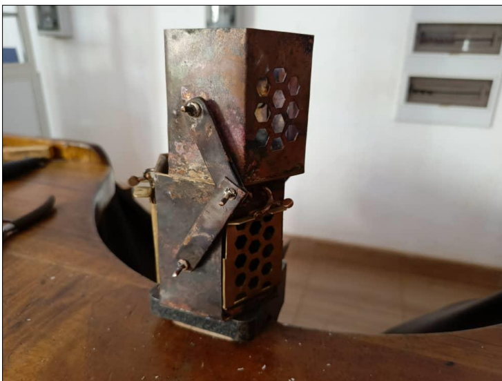
Fig 15: Both compartments riveted (Studio work, 2025)
