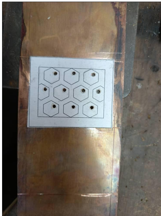
Fig 5: Drilling the template of the honeycomb (Studio work, 2025)
