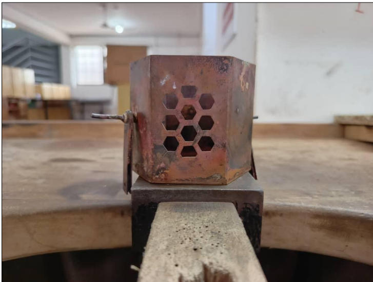
Fig 14: Riveting is done to support the movement of compartments (Studio work, 2025)
