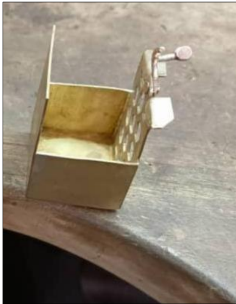
Fig 9: Riveting the lock on the drawer (Studio work, 2025)
