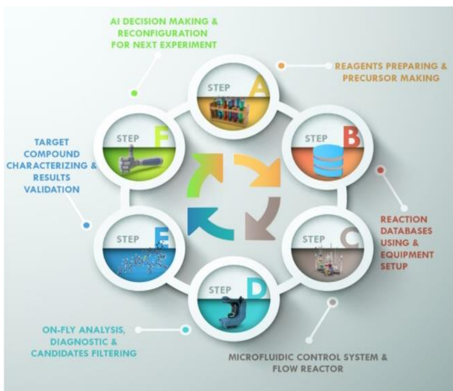
Fig 2: Fully automated closed-loop self-driving laboratory (Soldatov, et al. , 2021).
